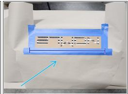
⚠ It's recommended to use thick packing paper or newspaper to masking the entire intercooler. Sufficient coverage is required or paint overspray **WILL** occur
