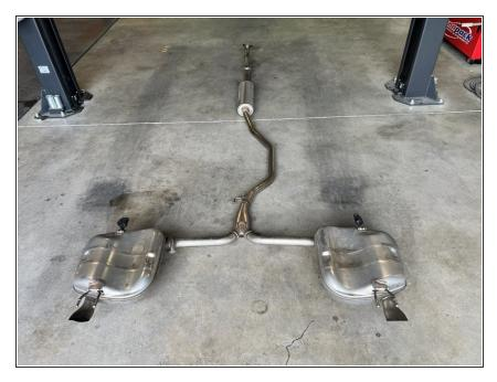
• With the exhaust unbolted and removed from the hanger supports, remove from the car and set aside
