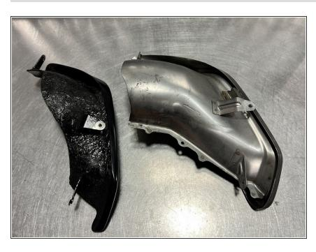
Identify the correct passenger side shroud as shown
