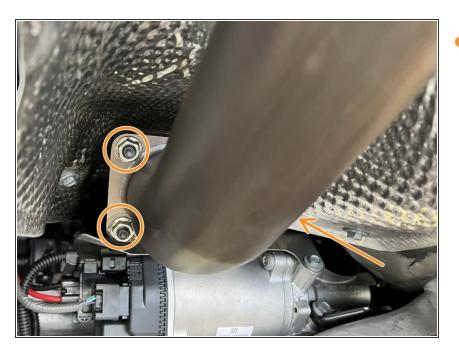
Torque the three (3) OEM nuts to 32 ft-lbs using the 14mm socket and 3/8 torque wrench
