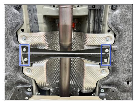
• Reinstall the 4x 12mm bolts for the chassis brace and torque to 20 ft/lbs
