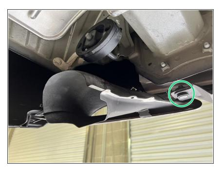
Use a flathead screwdriver or panel removal tool to remove the push clip and set aside for later
