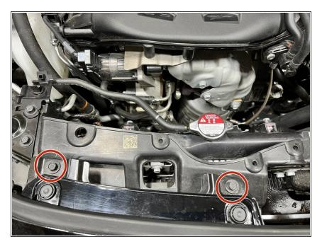
Locate the 2x 10mm bolts and remove them from the car. You will not reuse these bolts later
