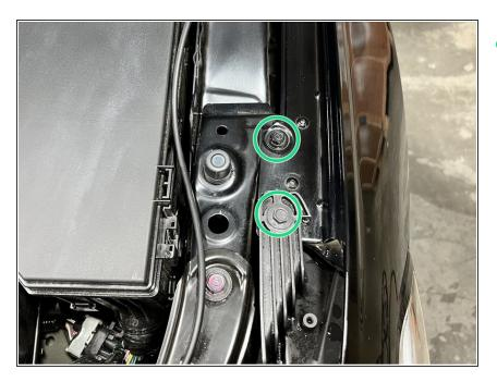
Use 3/8" ratchet and 10mm socket to remove the two (2) 10mm bolts
