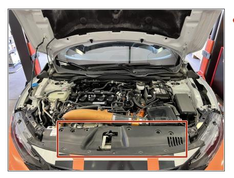
Open the hood to access the OEM radiator shroud
