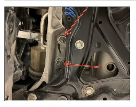
Using a 12mm socket, reinstall the (2) bolts to secure the front pipe support to the chassis
