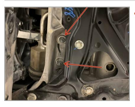
Using a 12mm socket, reinstall the
