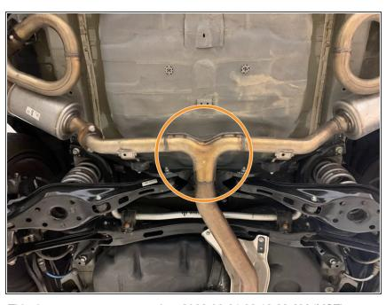
Using a transmission jack, floor jack, or a friend support the OE exhaust in the marked area
