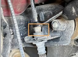
⚠ It is critical to use a Line Wrench to loosen the brakeline connection. Using the open end of a standard wrench may round the nut on the OE brake line
