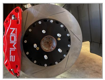
This completes the installation of the physical BBK. It's now necessary to bleed the brakes and bed the brake
