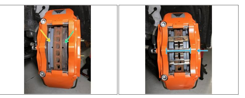
Install the new brake pad into the caliper as shown
