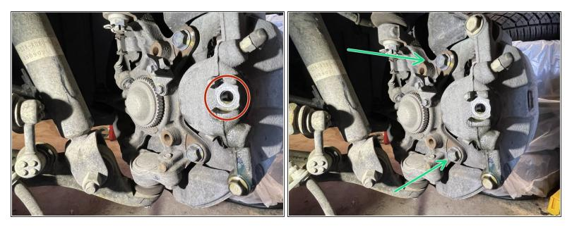
Disconnecting the brakeline will allow brake fluid to leak from the hard brakeline mounted to the chassis and the rubber brakeline on the caliper. Use a rag to catch drips
