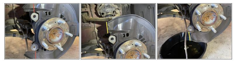
A Trimming of brake dust shields is required to accommodate the caliper brake bracket
