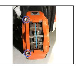
A Rotor installation may have put dirt/grease on rotor faces - clean rotor with brake clean spray and clean rag
