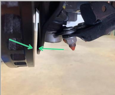
Check the clearance between the rotor and the dust shield
