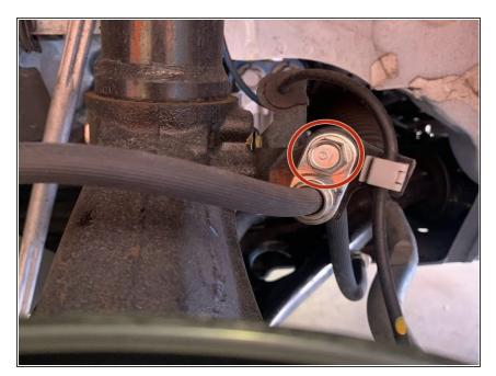
Use a 12mm socket and ratchet to remove the bolt shown with red circle
