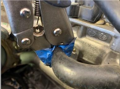
A small amount of water and coolant will spill out. Prepare the area with paper towels
