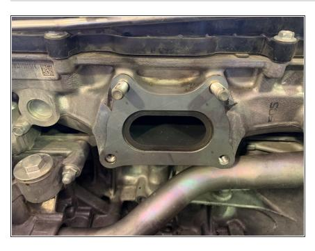
Install the provided turbo manifold gasket as shown
