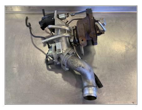
Remove the turbo assembly from the car and place on a workbench
