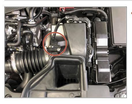
Unplug the MAF sensor by pushing down on the tab (red circle) on top of the wiring connector
