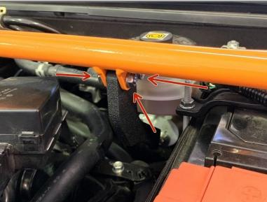
Tighten both sets of M6 hardware using either two 10mm wrenches or one 10mm wrench and a 10mm socket with a ratchet, tighten until snug (24-48 in-lbs)
