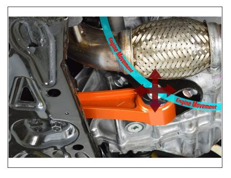
A performance rear motor mount by design reduces engine movement to mitigate unwanted wheel hop, slow throttle response, and torque steer - the by-product of this is increased NVH (Noise, Vibration, Harshness) that is transmitted to the vehicle cabin
