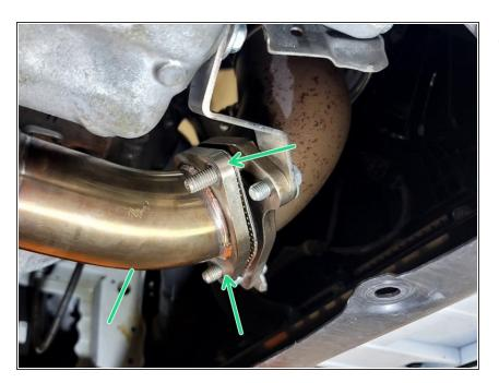
Reposition front pipe over the downpipe studs as shown
