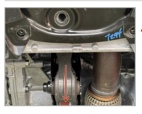
Pull the motor mount down a little bit and slide the OE Motor Mount toward the front to take it out
