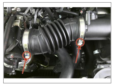
Reinstall accordion intake tube and tighten clamps with 5.5mm socket
