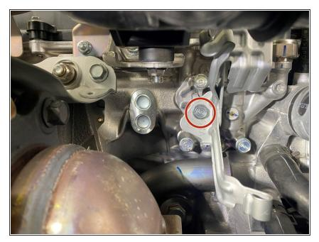
Bolt the secondary O2 sensor wire harness support bracket back in place. Torque bolt to 80 in-lbs.
