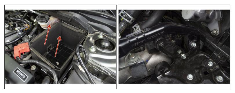
Remove the battery foam and tray case to reveal the battery bracket.
