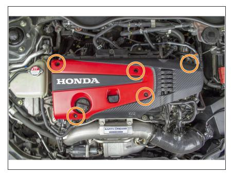
Align the engine cover on the engine, and install the five 10mm bolt with a 10mm deep socket and ratchet
