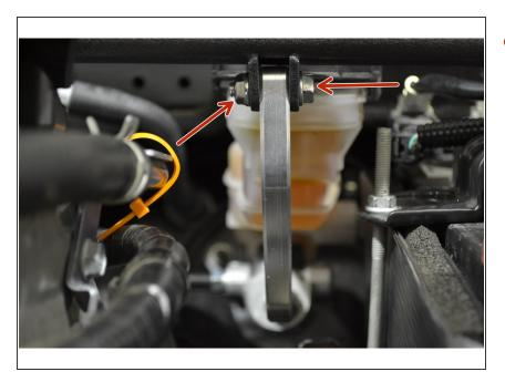
With the brake brace foot adjusted, tighten the M6 bolts and nuts installed earlier using either two 10mm wrenches or one 10mm wrench and a 10mm socket with a ratchet, tighten until snug (24-48 inlbs)
