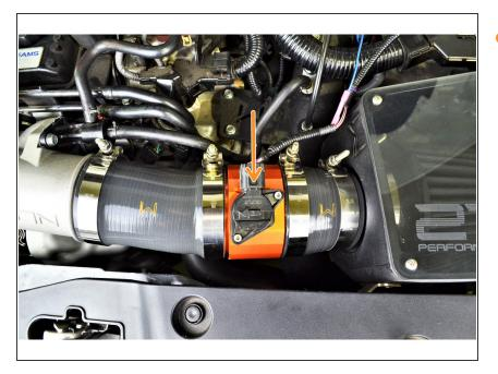
Connect the wiring harness to the MAF sensor as shown
