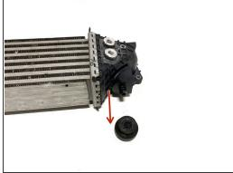
Remove the two (2) OEM rubber mounts from the bottom of the intercooler
