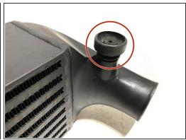
Install the rubber mounts onto the bottom mounting pegs of the 27WON intercooler as shown
