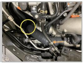
⚠ In this process try not to disrupt the assembly between the hot side pipe and turbo outlet silicone.
