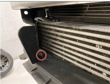
Use a flathead screwdriver to remove the two (2) push clips
