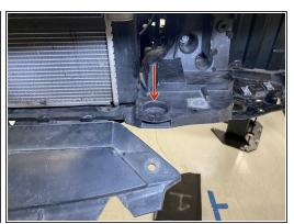
The rubber mounts will fit into the mounting pockets shown with the red arrows
