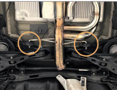
While supporting the rear of the muffler section, insert both forward hangers as shown
