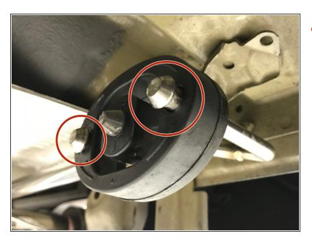
Verify that the bead of the hanger rods are through the dual rod rubber hangers as shown
