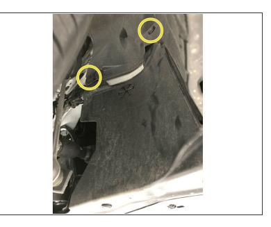
The images in this step show the push clips on the side of the under tray. These are labeled with the arrows in the previous step
