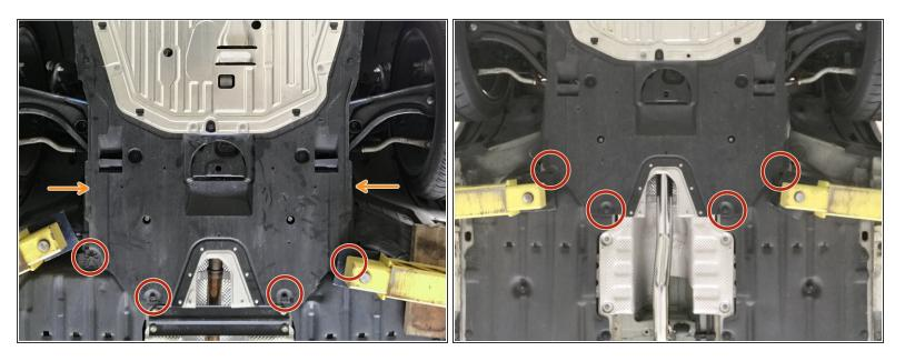
Re-install the 10mm bolts with a 10mm socket & torque wrench. Torque to 8-12 ft-lbs
