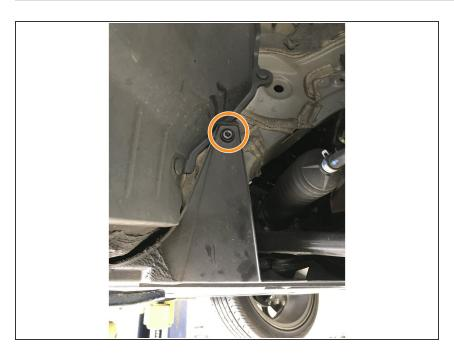
Re-install the push clips at each side of the undertray
