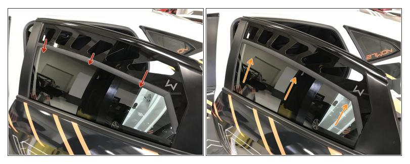
Without moving the window, place your fingers in the vents as shown and push the rubber molding & window vent down slightly to align and fit over the window edge
