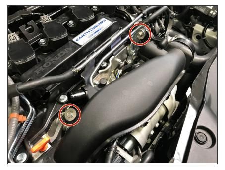
Use a 10mm socket & torque wrench to install the two (2) TIP mounting bolts. Torque to 8-10 ftlbs
