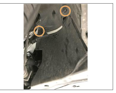
Use large flat head screw driver to remove push-clips on each side of skidtray
