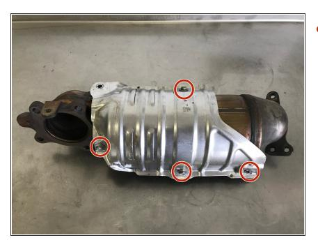
Use a 10mm socket & ratchet to remove the four (4) bolts
