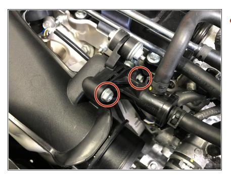
Use a 10mm socket & torque wrench to install the two (2) 10mm bolts. Torque to 8-10 ft-lbs
