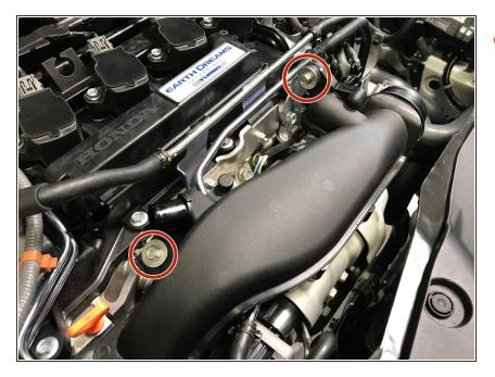
Use a 10mm socket & ratchet to remove the two (2) TIP mounting bolts
