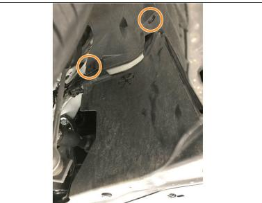
Install the remaning six (6) push-clips on each side of the skidtray
