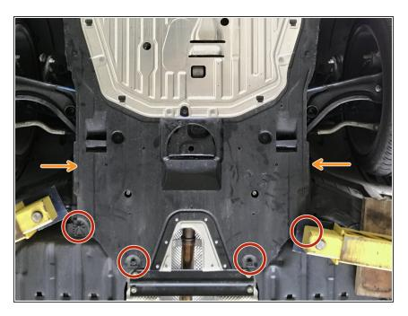
Re-install the 10mm bolts with a 10mm socket & torque wrench. Torque to 8-12 ft-lbs
