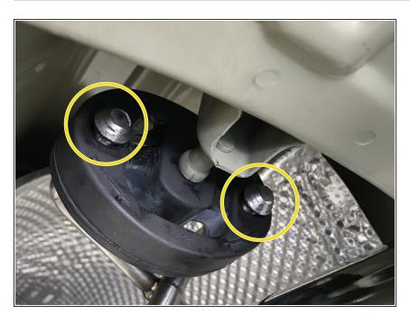
Re-position the rubber hanger rearward so it is against the hanger rod beads
