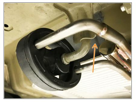
Verify that the hanger bar is not contacting the chassis. Move the muffler section rearward if the hanger bar is very close or touching the chassis
