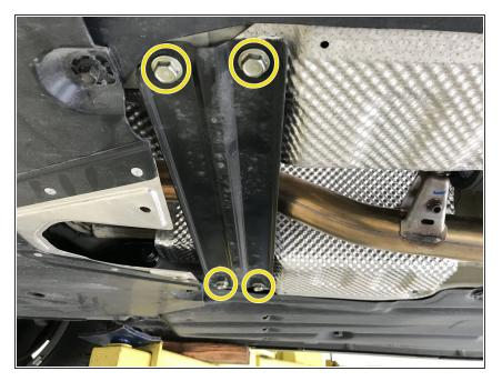
Re-install the cross member. Use a 14mm socket & torque wrench to torque the bolts to 25-35 ft-lbs
