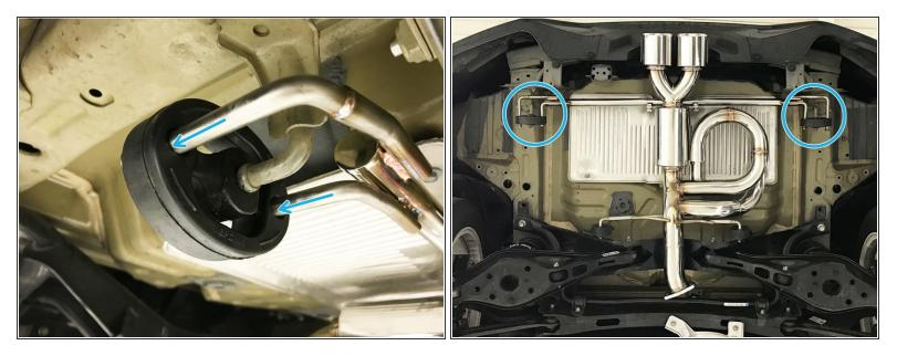
Then raise the rear end of the muffler section up and insert both rearward hangers
