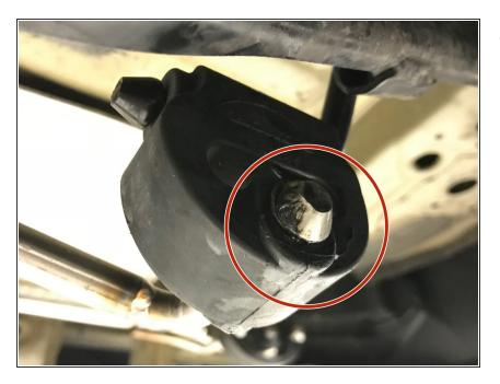
Verify that the bead of the hanger rod is through both forward rubber hangers as shown
