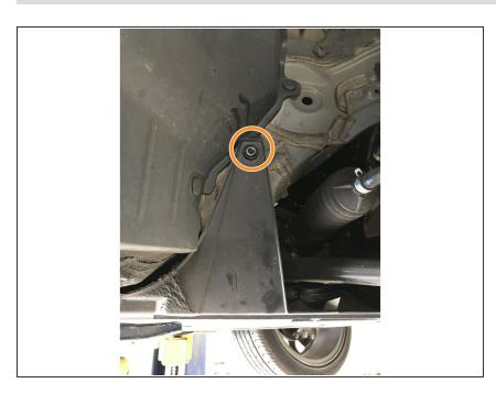
Re-install the push clips at each side of the untertray
