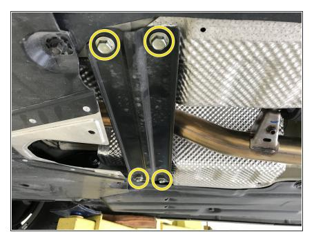
Use 14mm socket & ratchet to remove the 4 bolts holding the cross member
